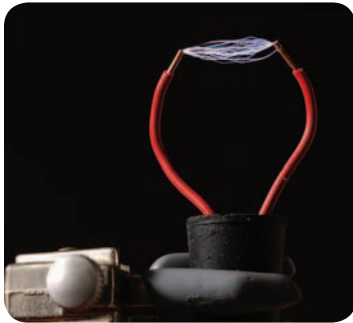
FIGURE 16.25 Dielectric breakdown in air. Sparks are produced when a large alternating voltage is applied across the wires by a high-voltage induction coil power supply.
