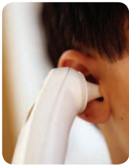
FIGURE 11.14 A radiation thermometer measures a patient's temperature by monitoring the intensity of infrared radiation leaving the ear.
