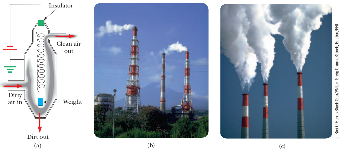
FIGURE 16.12 (a) A schematic diagram of an electrostatic precipitator. The high voltage maintained on the central wires creates an electric discharge in the vicinity of the wire. Compare the air pollution when the precipitator is (b) operating and (c) turned off.
