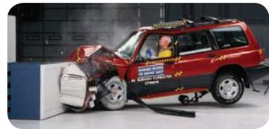
FIGURE 6.4 (Example 6.2) (a) This car’s momentum changes as a result of its collision with the wall. (b) In a crash test (an inelastic collision), much of the car’s initial kinetic energy is transformed into the energy it took to damage the vehicle.
