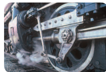
FIGURE 13.10 The drive wheel mechanism of an old locomotive.
