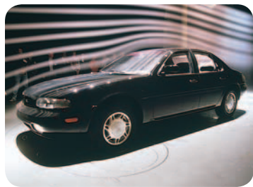
FIGURE 9.26 An illustration of streamline flow around an automobile in a test wind tunnel. The streamlines in the airflow are made visible by smoke particles.
