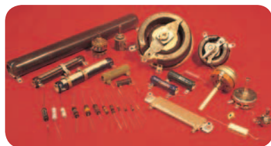
An assortment of resistors used for a variety of applications in electronic circuits.
